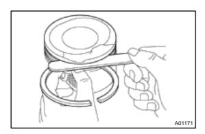
(b) Inspect the piston ring groove clearance.
