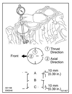
Inspect the cylinder bore diameter. Using a cylinder gauge, measure the cylinder bore diameter at positions A, B and C in the thrust and axial directions.
