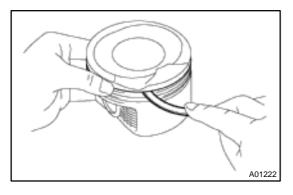
(b) Using a groove cleaning tool or a broken ring, clean the piston ring grooves.
