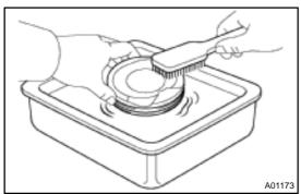
(c) Using a brush and solvent, thoroughly clean the piston.NOTICE:Do not use a wire brush.
