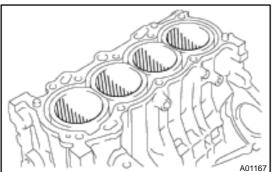
(b) Visually check the cylinder for vertical scratches. If deep scratches are present, replace the cylinder block.
